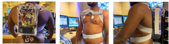
Figure 2. Back, front, and side profiles of the wearable harness on a surgeon volunteer at the STRATUS Center for Medical Simulation.
