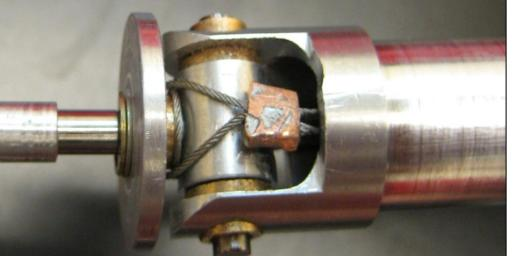
These bolts are loosened to create tension in the cables
