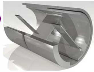
Cross-section rendering through a C'Flex flexural pivot bearing (see www.c-flex.com Special thanks to William R. Herbstritt of Pageboys Web Design for the rendering!)
